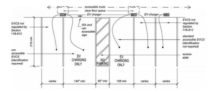
Figure 3: 26 EVCS = three accessible EV Spaces required
